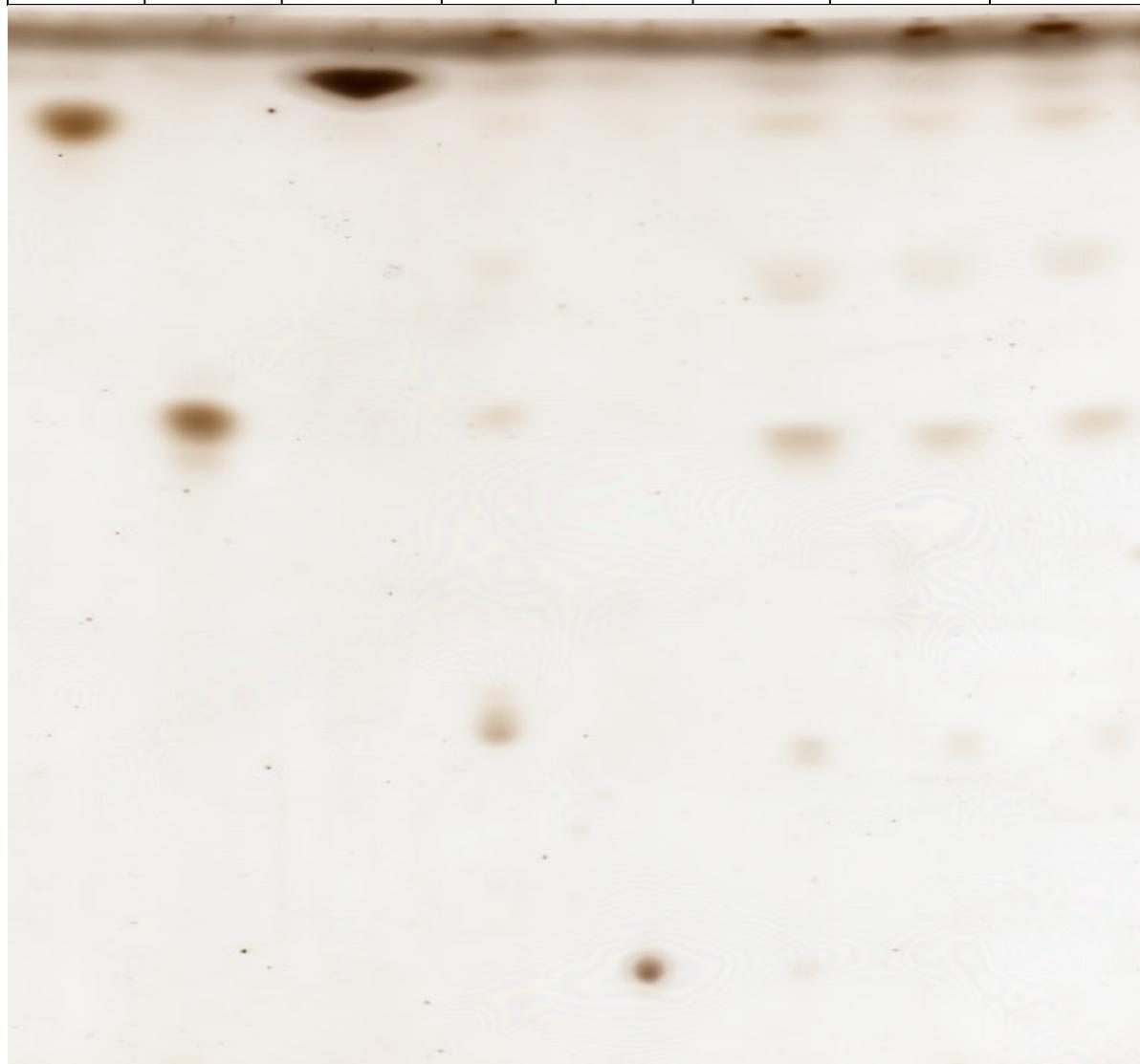
**Figure 1.** Thin-layer chromatography plate of lipids extracted by ethanol, chloroform and diethylether. Standards: Monogalactosyldiglyceride (MGDG), Digalactosyldiacylglyceride (DGDG), L- $\alpha$ -phospahtidylcholine (PC), L- $\alpha$ -lysophospahtidylcholine (LPC).
