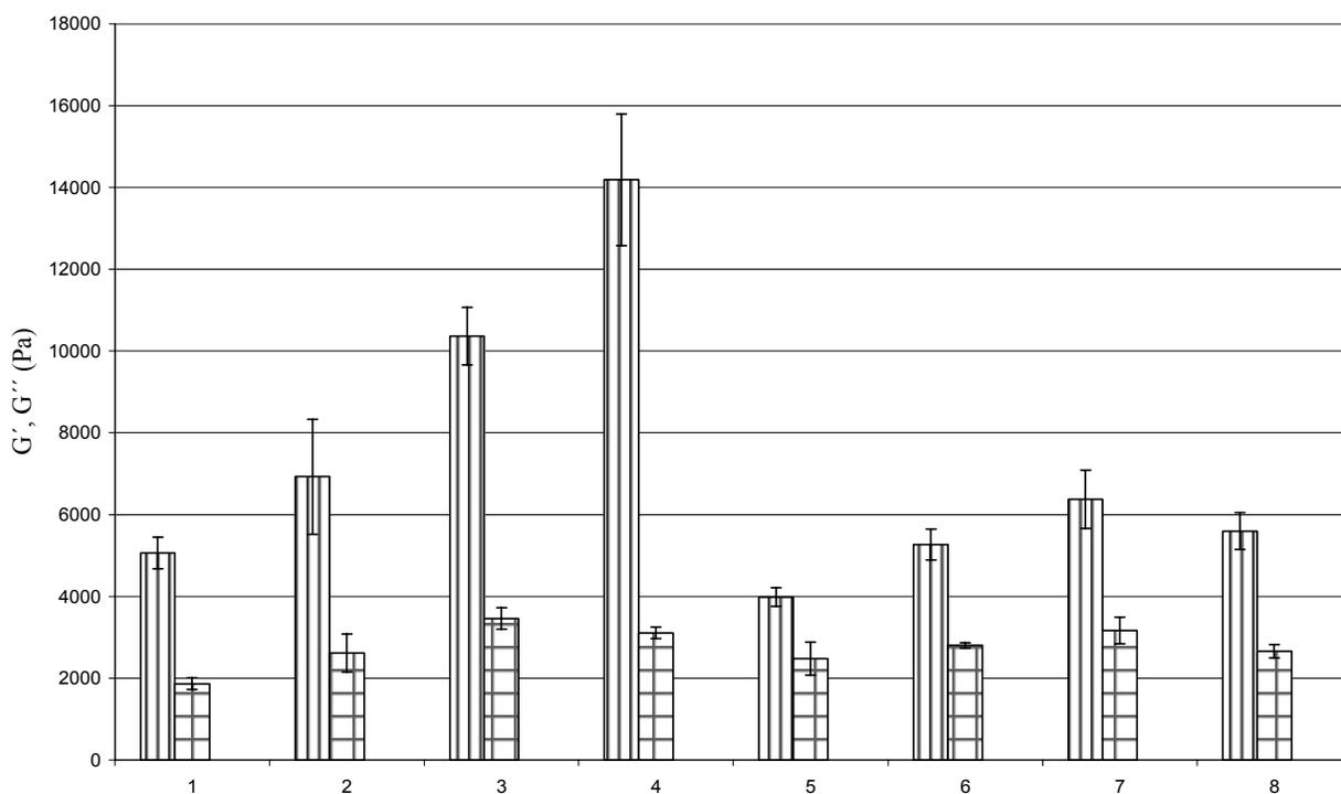
**Figure 3.** Storage modulus ( $G'$ , striped) and loss modulus ( $G''$ , squares) for dough and gluten at a frequency of 1 Hz,  $T=25^\circ\text{C}$ . The water content of the dough was 46.5%. Doughs made with native flour (1), and flours where the lipids had been removed by diethylether (2), chloroform (3) and ethanol (4). Gluten from doughs made with native flour (5), and flours where the lipids had been removed by diethylether (6), chloroform (7) and ethanol (8).
