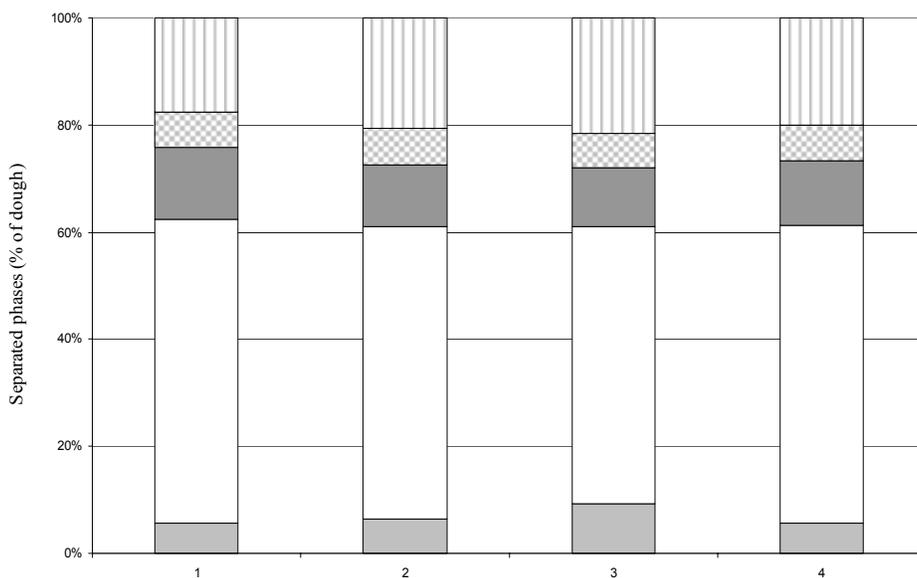
**Figure 2.** Separation of wheat flour dough (water content 46.5 % (w/w)) by ultracentrifugation. Dough made with Kosack flour (1), and Kosack flour where the lipids had been removed by diethylether (2), chloroform (3) and ethanol (4). The separated phases are (from the top): liquid, gel, gluten, starch and unseparated dough.
