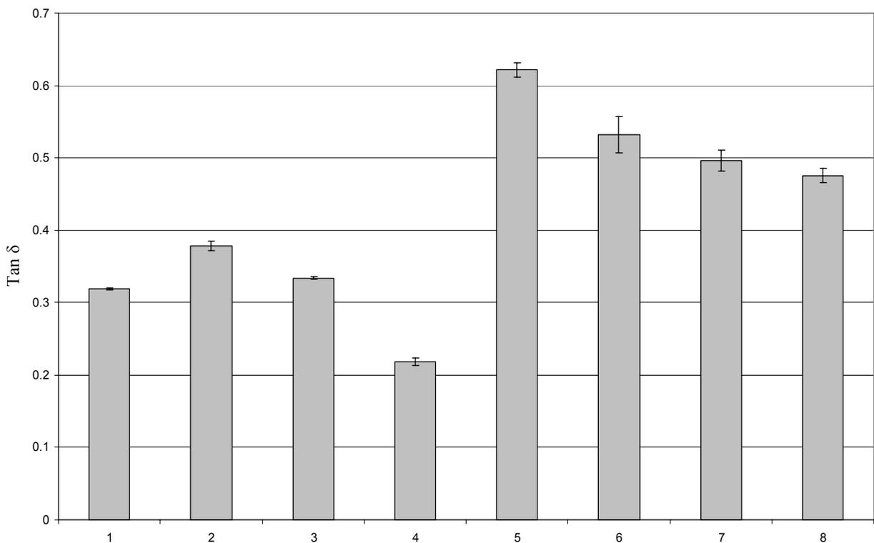
**Figure 4.**  $\tan \delta$  at a frequency of 1 Hz for doughs made of native flour (1) and of flours where the lipids had been removed by diethylether (2), chloroform (3) and ethanol (4) and of gluten prepared from doughs of native flour (1) and of flours where the lipids had been removed by diethylether (2), chloroform (3) and ethanol (4).
